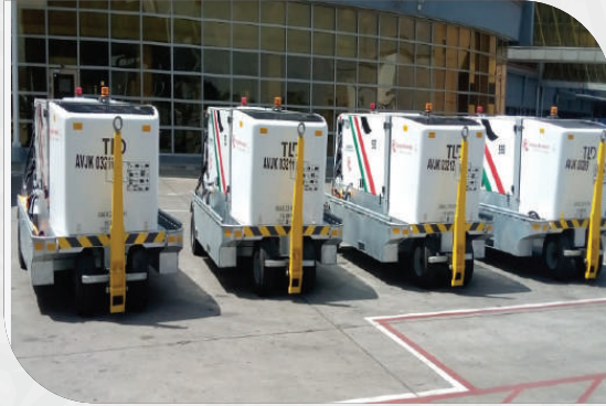
4 new Ground Power Units (GPU)
